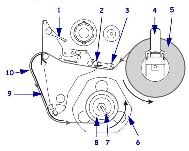
Figure 29 • Media Loaded in Rewind Mode
